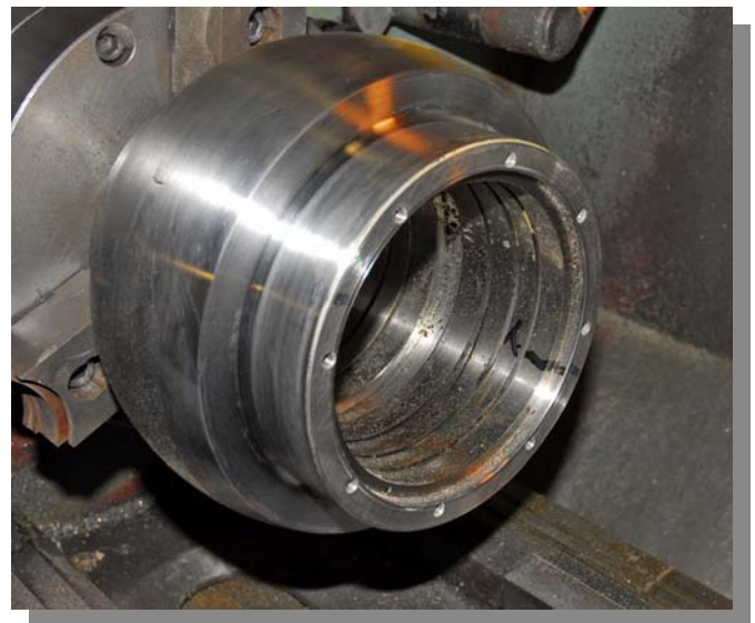
Doctor Bearing in the beginning of refurbishing process.
