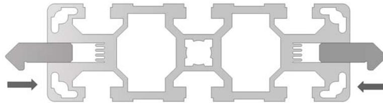
**Fig. 7:** Steel v-rails inserted in extruded or machined pockets containing fingers in an aluminum structure.
