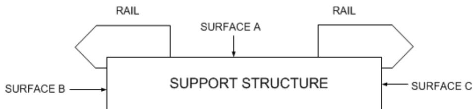
Fig. 3: The accuracy of v-roller rails is largely dependent on the flatness, straightness and parallelism of the surfaces to which they mount.
