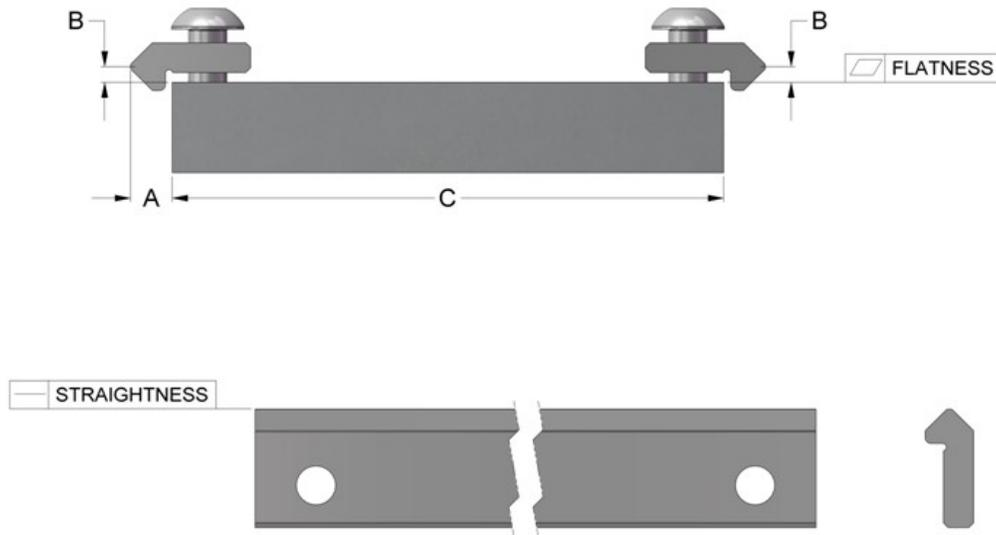
**Fig. 5:** Stack-up of tolerances affects the location tolerances of steel v-rail assemblies
