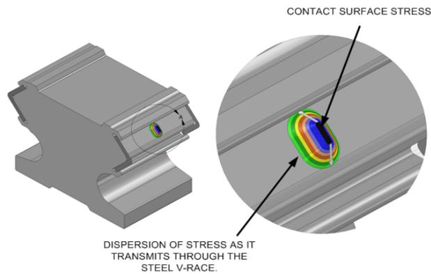
**Fig. 9:** Steel v-race shown transparent so that the dispersion of the contact surface stress as it progresses through the steel v-race can be seen.
