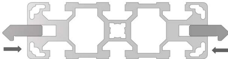
**Fig. 6:** Steel v-rails inserted into extruded pockets in an aluminum structure.
