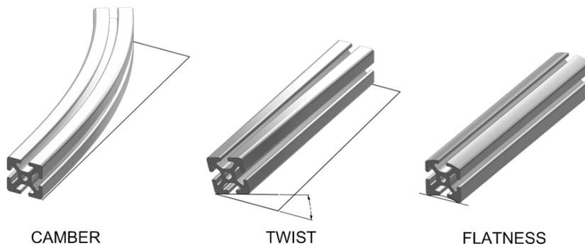
**Fig. 4:** Illustration of camber, twist and flatness.
